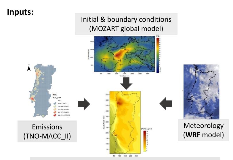
**CAMx** air quality model with PSAT (Particulate Source Apportionment Tool)
